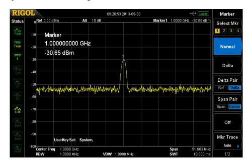
Note that the marker now shows -30dBm for the amplitude. This is due to the probe attenuation factor.
