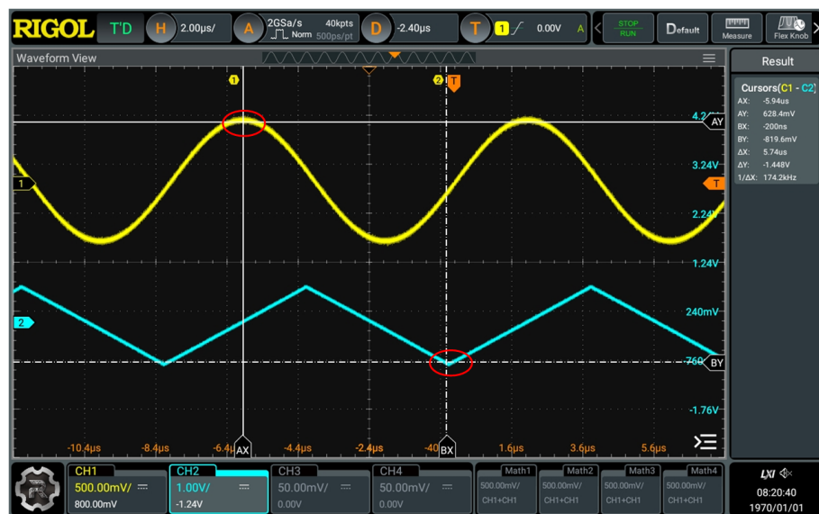
Figure 10.13 Track Measurement (after Horizontal Expansion)
